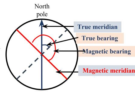
**True Meridian:** the line of intersection of the earth surface by a plane containing a North pole, South pole and observers position is called True meridian or geographical meridian. Geographical meridian are not parallel to each other. These converge to a point in northern and southern hemisphere.
