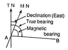
Determination of true bearing and magnetic bearing:
